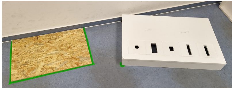
Figure 3.5: left: 0cm-Table with arbitrary surface (approx. 1cm thick); right: PPT-Table which is a standard 10cm-Table with cavities
