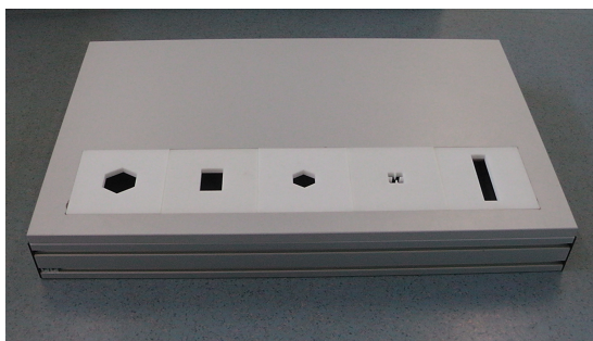
(a) The PPT platform including five cavity tile.
